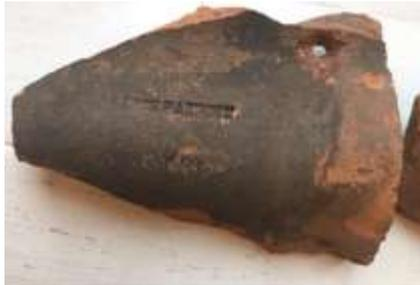
**The handmade clay roof tile stamped “Sealy’s Patent**
